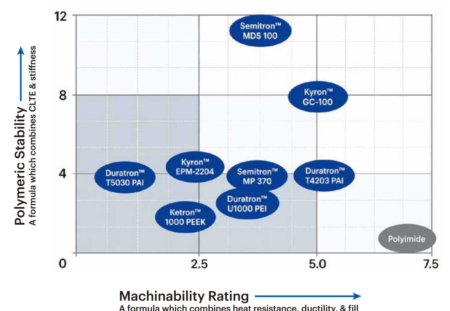
Test socket material selection grid Polymeric stability vs. machinability of fine features
